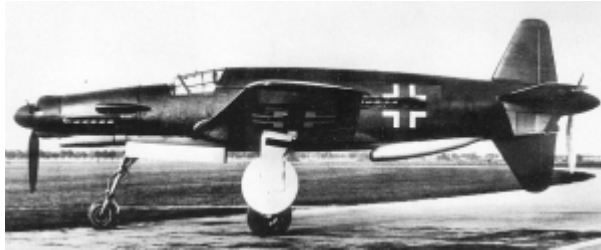
Do 335V-1 with chin oil cooler and circular mainwheel doors. (photo, Dornier)
