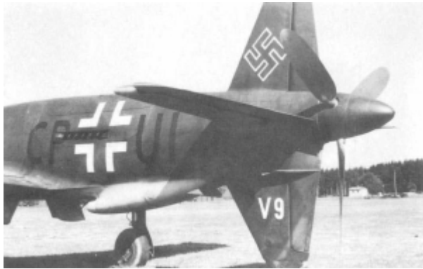
Rear propeller installation on Do 335V-9 CP+UI 23009. (photo, Dornier)
