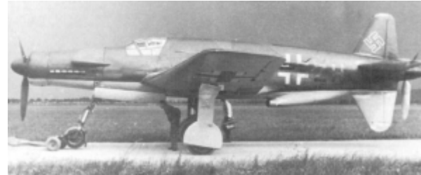
Do 335V-3 T9+ZH with revised nose shape and mainwheel doors. (photo, Dornier)
