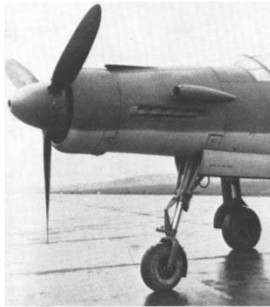
Nose engine installation (photo, Dornier)
