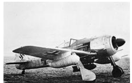
Fw 190 G-1 showing the ETC 250 bomb rack, carrying a 250 kg (550 lb) bomb, and the underwing drop tanks on VTr-Ju 87 mounts.
