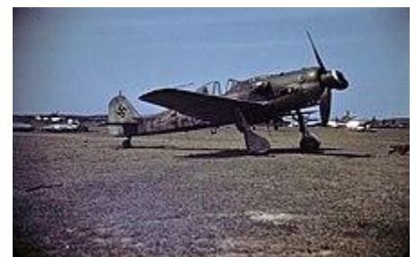
This captured Fw 190 D-9 appears to be a late production aircraft built by Fieseler at Kassel. It has a late style canopy; the horizontal black stripe with white outline shows that this was a II. Gruppe aircraft.
