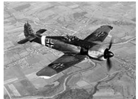
A captured FW-190A. The aircraft was repainted while being tested by the USAAF. The markings are incorrect in size, proportion, and location. This plane has the cowling extension (see wing root), and so is an A-5 or later model. If its cowling machine guns were faired over at the factory, this may be an FW-190G.
