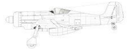
The Fw 190C V18 prototype, with large ventral "pouch" fairing for the turbocharger installation and broader-chord vertical fin/rudder.
