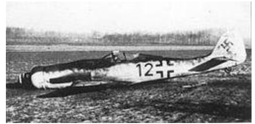
A Fw 190D-9 of 10./JG 54 Grünherz , pilot (Leutnant Theo Nibel), downed by a bird which flew into the nose radiator near Brussels on 1 January 1945.
