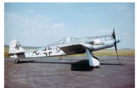
A side view of the NMUSAF 's D-9. One can easily distinguish the D-9 model from earlier variants by the extended nose and tail sections, in addition to the exhaust manifolds located near the base of the engine cowling.
