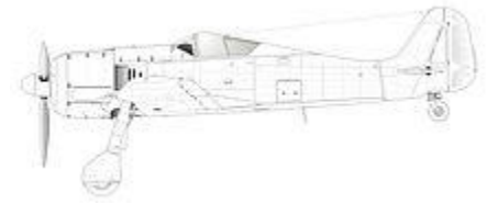
Side-view of Fw 190 A-2; the most notable change over the A-0 was the addition of three vertical cooling slits on the engine cowling, just forward of the wing.
