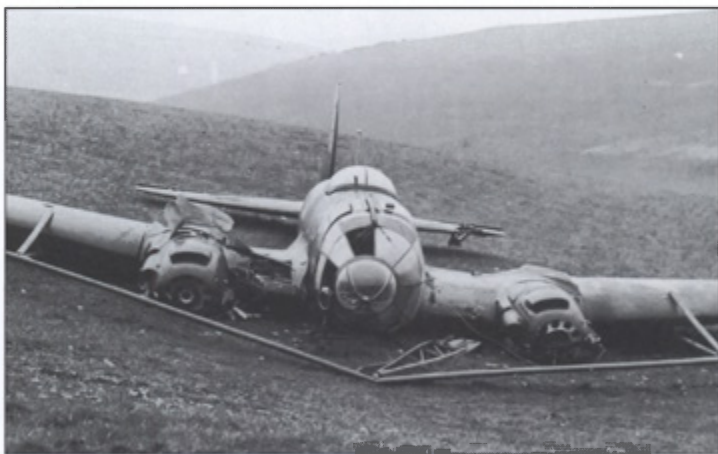
He 111H-8 '1G+ZM' of 4./KG 27 is seen here spread-eagled on a Dorset hillside on the morning of 23 May 1941 after its involuntary arrival the evening before. The bomber's elaborate balloon-cable fender aroused sufficient interest for the machine to be taken to RAE Farnborough for further examination
