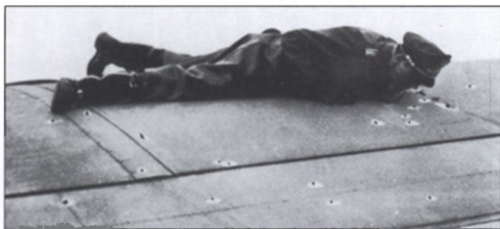
The Heinkel Gruppen in Poland suffered at the hands of enemy fighters and ground fire alike. These appear to be machine gun bullet entry holes, which would suggest a fighter attack from above. Although not manoeuvrable enough always to be able to take effective avoiding action, the He 111 was sturdy and could usually absorb such damage as this and much more
