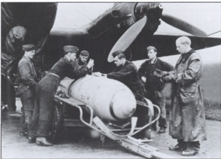
An armourer sets the fuse for the second of the two SC 1000 bombs to be loaded onto the external bomb racks of this He 111H
