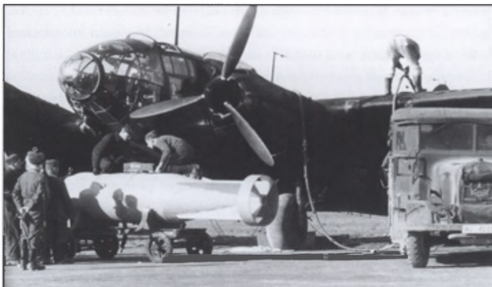
While a member of the groundcrew (right) tops up the port outer fuel tank, a group of armourers begin the tricky job of hoisting an SC 2500 'Max' onto Ill./KG 26's '1H+PT'
