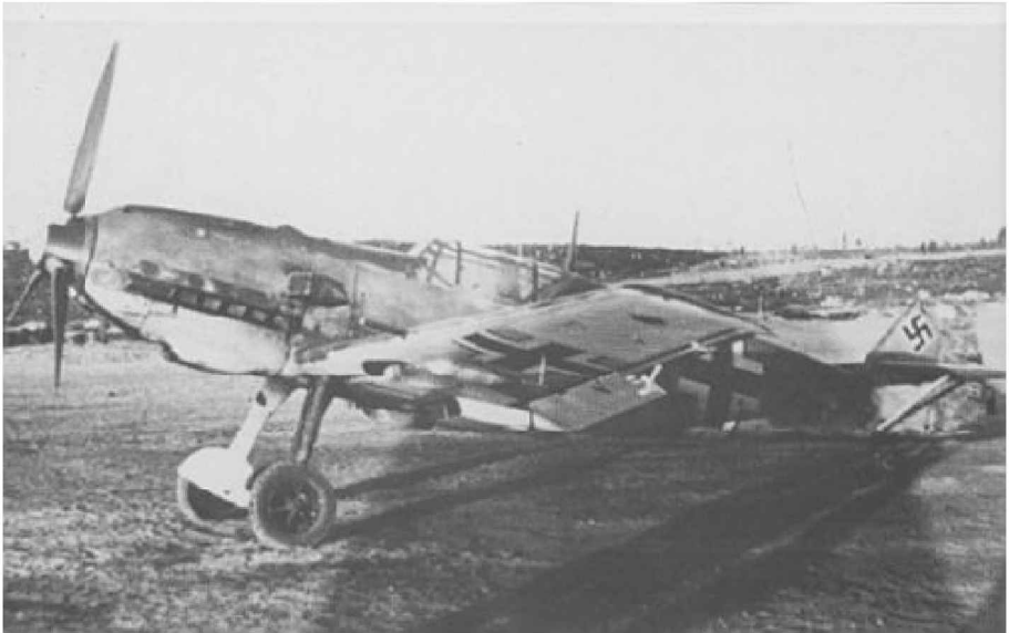
A Bf 109E of 1./JG 77, Rovaniemi, summer 1941. This aircraft is an E-3 upgraded to E-7 standards. The lower wing tips are painted yellow to denote the eastern front. The yellow spinner tip would also indicate that the machine belonged to the 3 Staffel , (via B. Barbas)
