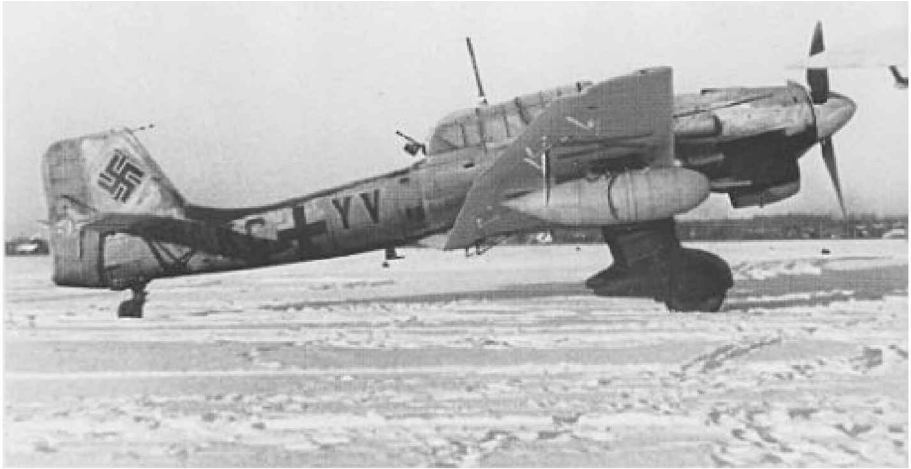
A Ju 87R-2 with Stammkennzeichen KC+YV on a transfer flight at Helsinki Malmi airport. It continued its journey on 11 January 1943 to Pori, on the way to St.G 5. The white distemper was roughly applied with a wide brush. (A. Korhonen)
