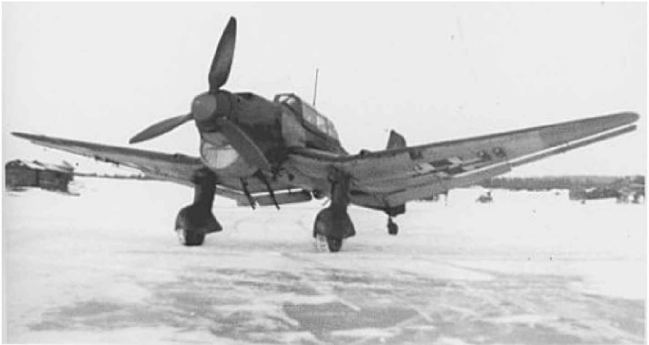
A Ju 87B-2 of 2./St.G 5 being refuelled at Alakurtti in spring 1942. The old unit designation L1 can still be distinguished on the rear fuselage. The SC 50 bombs in the wing racks were fitted with extended fuses and used against troops and columns. (Author's collection)
