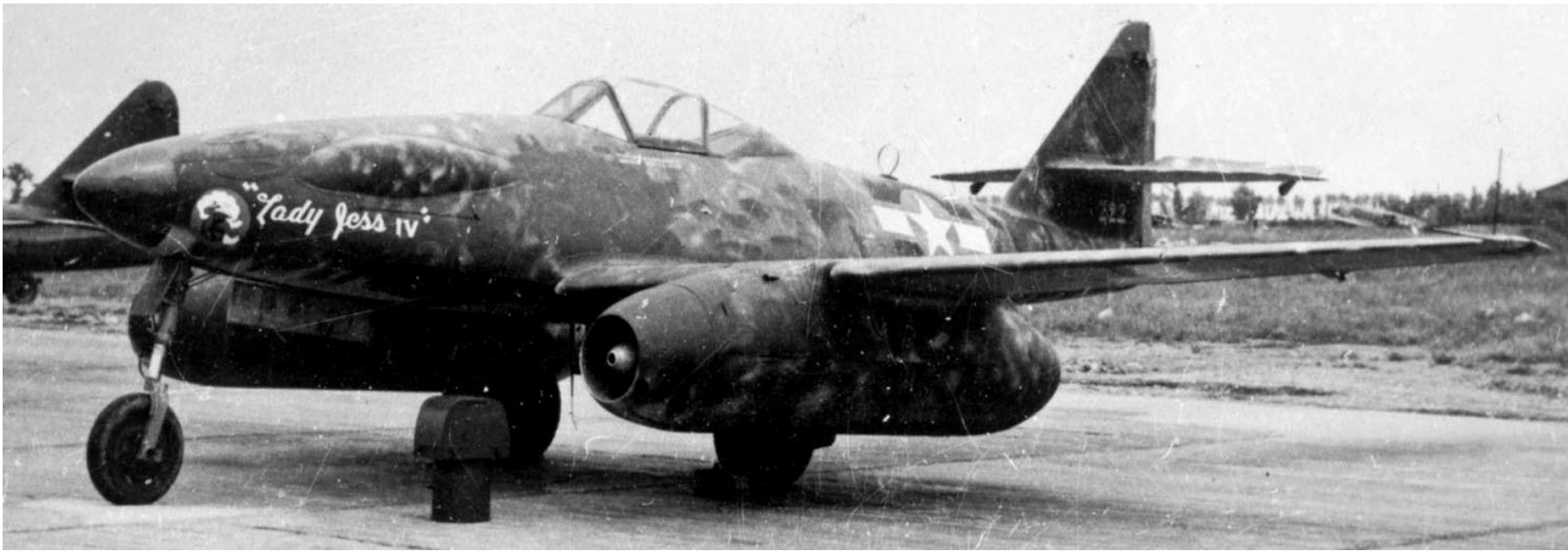
Messerschmitt Me 262A-1a/U3 (Wk. Nr. unknown), " White 30 ", reconnaissance version modified with bulges on the nose to accommodate film magazines for two Rb 20/30 cameras. U3 (Umrüst-Bausatz 3, Factory Modification Kit No. 3). Watson's Whizzers 222, " Marge ", later " Lady Jess IV ". It was flown by Capt Kenneth Dahlstrom. Artwork was painted on the nose with a picture of Donald Duck circling the globe on a jet engine, with "Watson's Whizzers" in print. " White 30 " was shipped to the USA on HMS Reaper . It was allocated FE-
