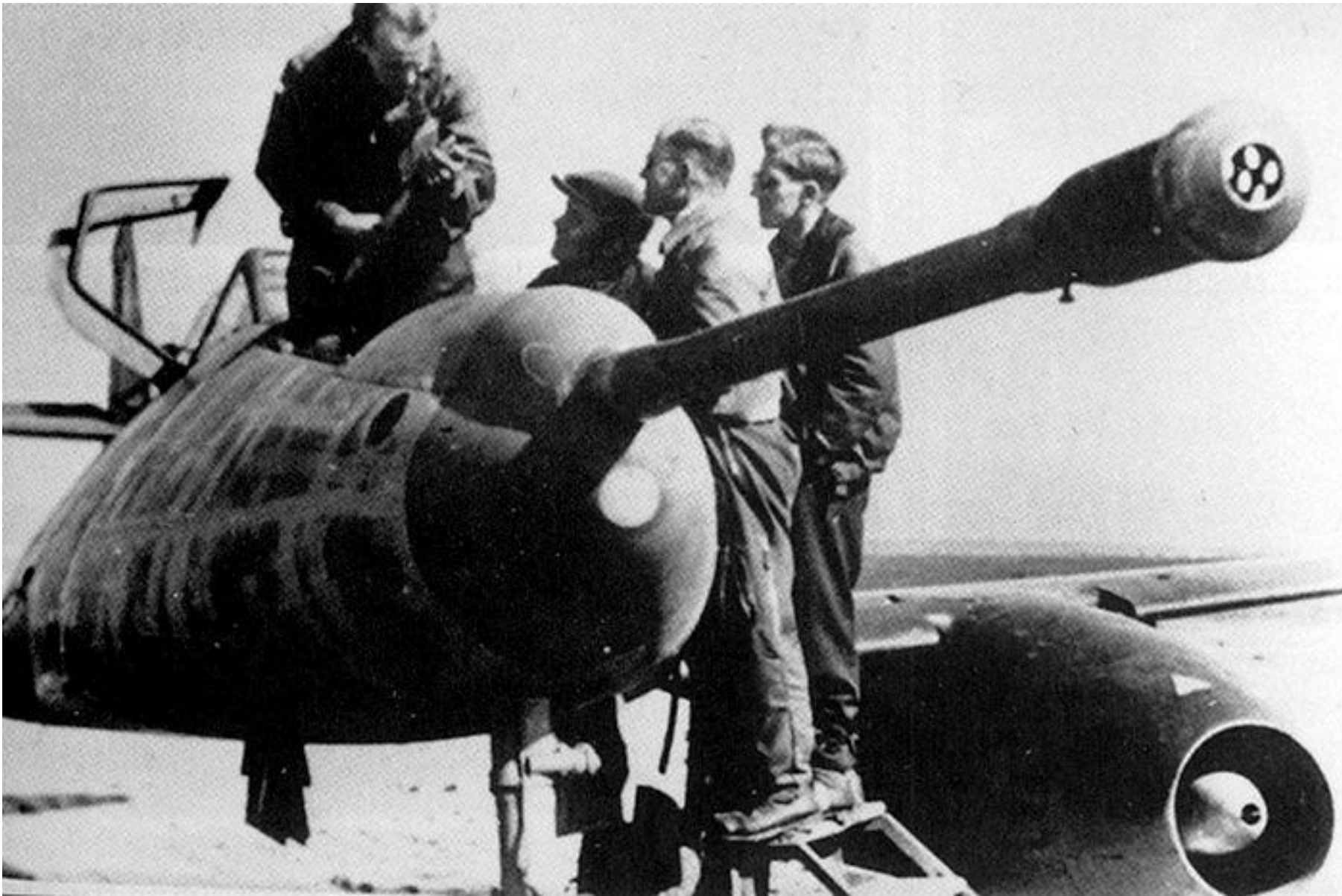
Messerschmitt Me 262A-1a/U4, (Wk. Nr. unknown), "Pulkzerstörer", bomber destroyer version armed with one 50-mm Mauser Mk. 214 cannon. USAAF "Feudin 54 A.D Sq". Possibly shipped to the USA, fate unknown. (USAAF Photos)
