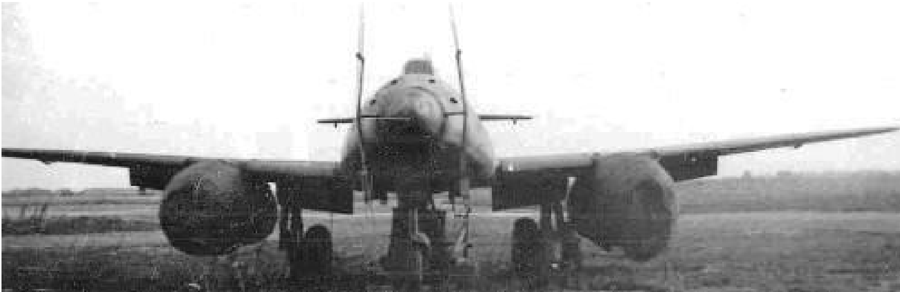
Messerschmitt Me 262B-1a/U1 (Wk. Nr. 111980) "Red 12" , 10./NJG11, two-seat trainer converted into a provisional night fighter version equipped with FuG 218 Neptun radar and Hirschgeweih (stag antler) eight-dipole antenna array. "Red 12" was flown by Lt Herbert Altner to Schleswig-Jagel, Germany, on 6 May 1945, where it was collected by the RAF. This aircraft was taken to England, and designated AM53. It was destroyed during a storm at Brize Norton in 1947. The remains were scrapped at Sealand in 1948. (RAF Photos)
