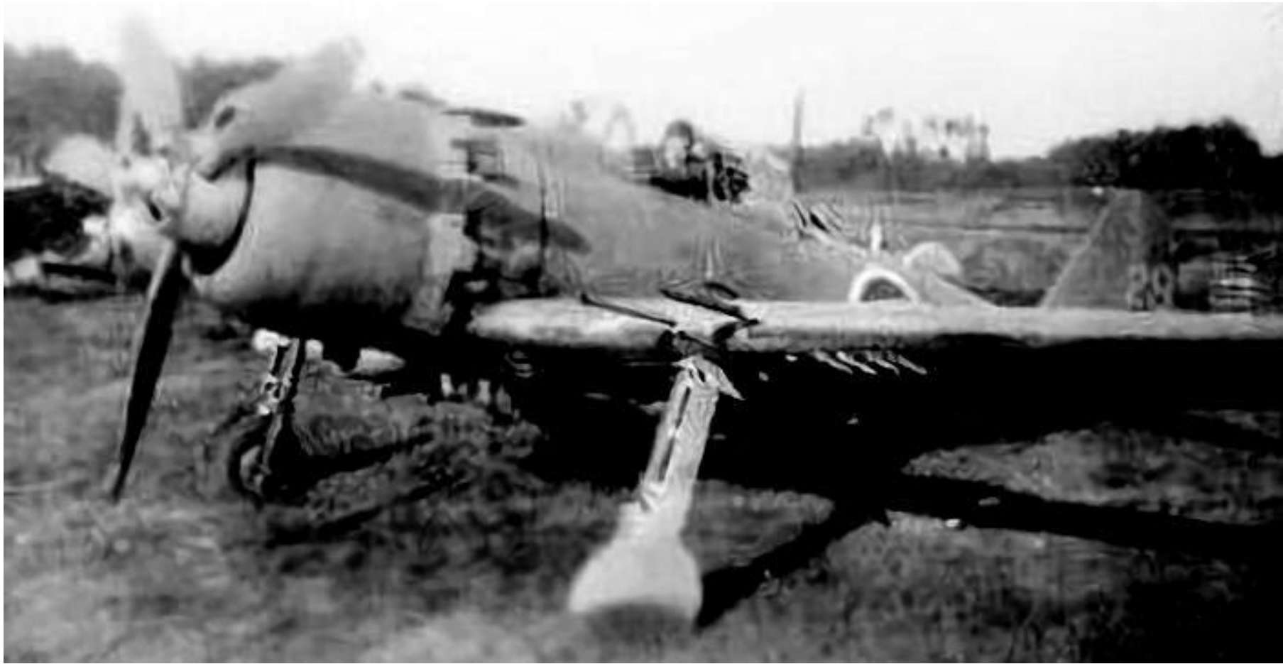
Mitsubishi A6M8 Model 64 Zero-Sen (Navy Type 0 Carrier Fighter), codename “Zeke”, with a Kinsae 64 engine. One of two prototypes completed. One was shipped to the USA and designated USAAF FE-311. This aircraft was scrapped at Park Ridge ca. 1950. (IJAAF Photo)
