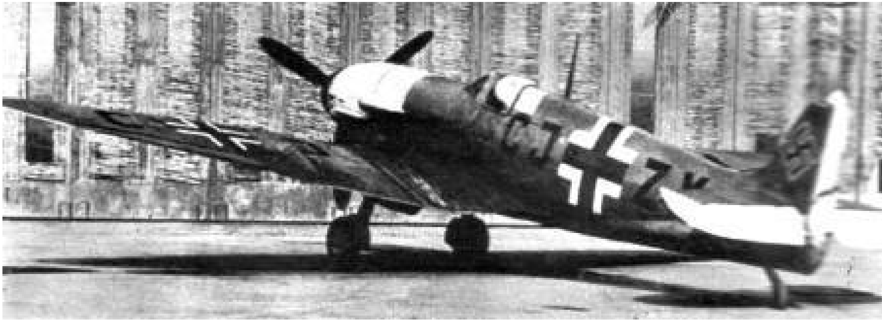
Supermarine Spitfire, coded CJ-ZY, captured British fighter re-engined with a German Daimler engine. (Luftwaffe Photos)
