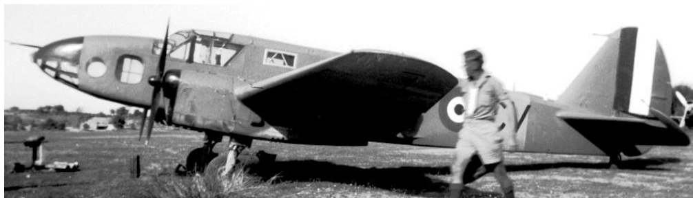
Caproni Ca.309 Ghibli (South Wind) reconnaissance. This Ghibli was captured by the RAAF in North Africa. Originally used for dropping flares, this aircraft was converted to transport personnel and flown by RAAF No. 3 Squadron. (Jim Kinnear Photo)
